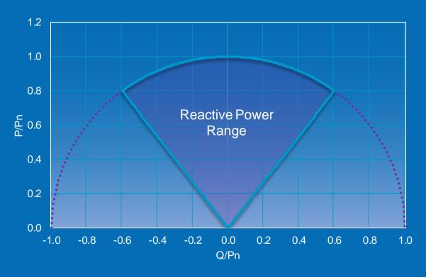
Reactive Power Range: [0.8<sub>lag</sub>,0.8<sub>lead</sub>] Max. Apparent Power: 100%Pn
